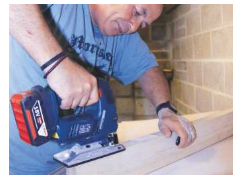
▲ Making a plunge cut on a worktop is easy with the GST 18V-LI B
